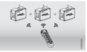
One transmitter can control one of a maximum of three pre-paired Demag DRC-MP radio receivers. The active radio receiver transfers the commands to the relevant crane. The transmitter can be switched between the receivers by pressing a combination of buttons.
